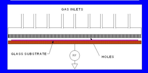
Fast and uniform gas feed for depositing amorphous silicon on very large glass substrates for displays (Applied Komatsu)
